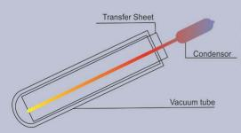
Heat pipes have a particularly strong heat conduction capacity. Using phase transition principle and capillary action, its heat conduction efficiency is higher. Water is Heated by the Heat Pipes rapidly.
